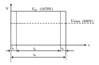
$\begin{array}{ll} t_3 \text{ , } t_4 & = 0.1s \\ t_p \text{ (Partial discharge } & = 1s \\ \text{measuring time)} & = 1.2s \end{array}$
